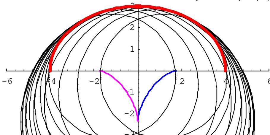
$$\begin{aligned} x &= A \cos^3 \varphi \\ y &= A \sin^3 \varphi \end{aligned}$$
